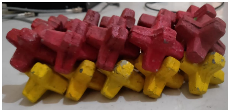
Fig. 1. Interlocking property of the Hexaloc concrete armor units
