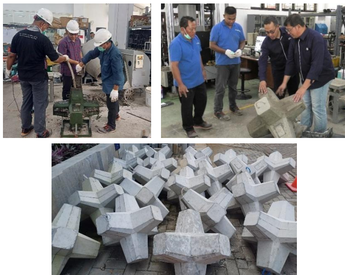
Fig. 3. Laboratory process for producing Hexaloc units
