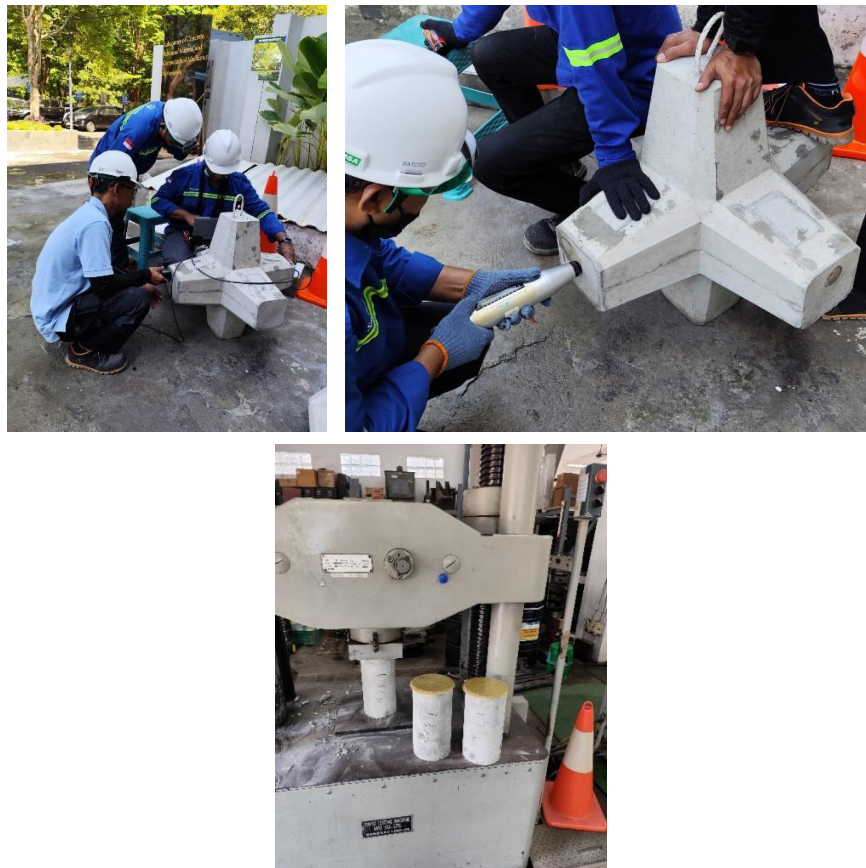
Fig. 4. UPV test, rebound hammer test, and compressive strength test of Hexaloc concrete samples.
