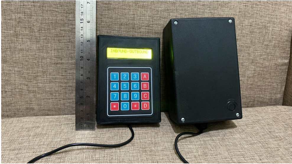
Fig. 4. Assembled IoT-based fish stock recording instrument.
