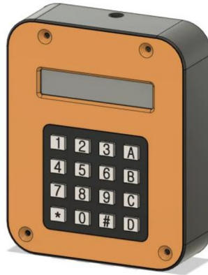
Fig. 1. Design of the assembled inbound–outbound fish data recorder.
