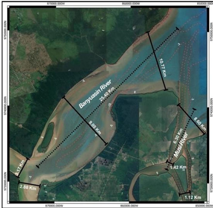
Fig. 3. Spatial morphology of the Banyuasin and Musi River Estuary. This map displays critical dimensions and bathymetric contours of the river systems, including the 25.40 km Banyuasin River stretch, to provide spatial context for hydrodynamic analysis.
