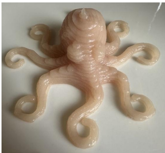
Fig. 1. Printed product at v=50 mm/s, V=55 mm 3 /s, D_n=1,4 mm, \phi=60\%
