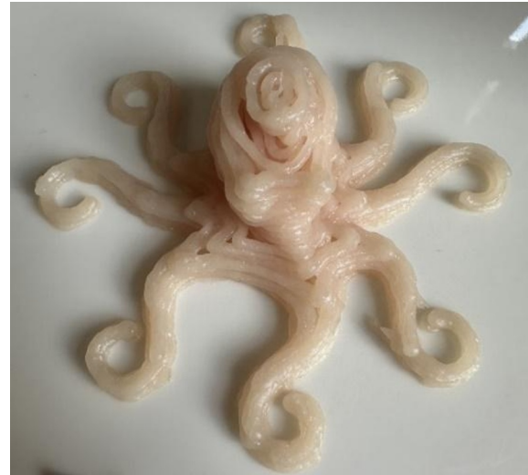
Fig. 2. Printed product at v=60 mm/s, V=50 mm 3 /s, D_n=1,6 mm, \phi=30\%
