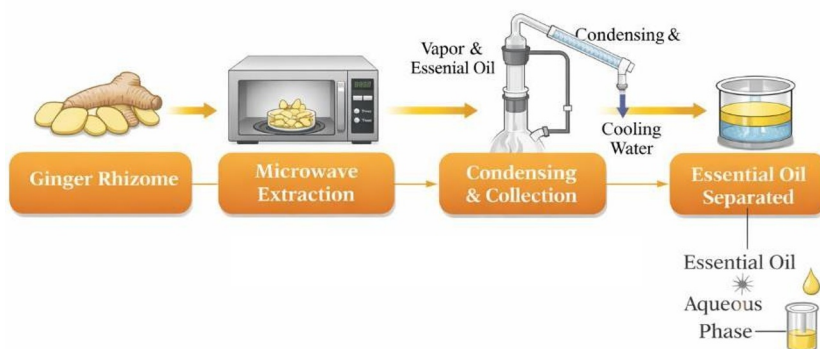
Fig. 2. Solvent Free Microwave Extraction Scheme
