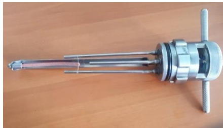
Fig. 2. Sample holder of Accoustic Emission Strandburner
