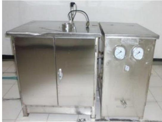
Fig. 1. Burn rate testing apparatus : Acoustic Emission Strand Burner (AES)
