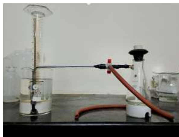
Fig. 2. Schematic of the customized water displacement setup used for hydrogen evolution measurements.
