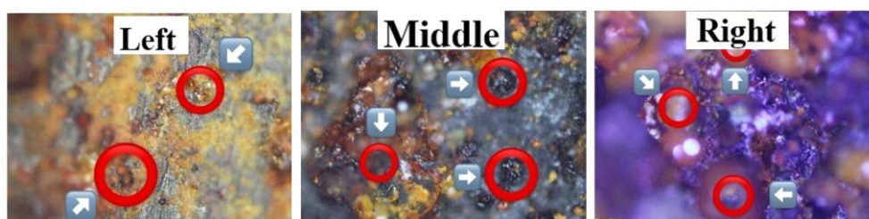
Fig. 5. Optical micrograph (20×Magnification) of the specimen in the absence of Psidium guajava leaf extract.
