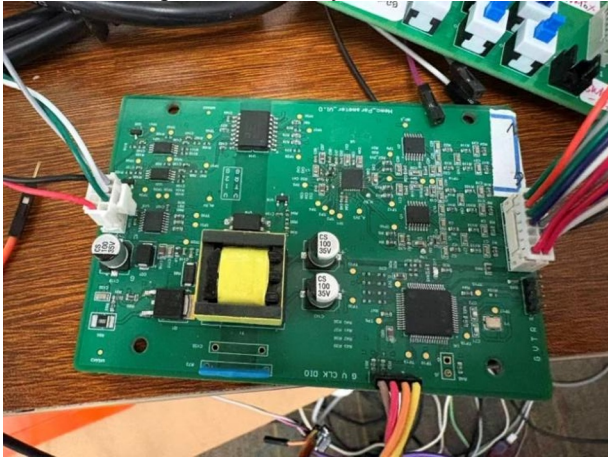
Figure 3. Main board of the hemodynamic monitoring module
