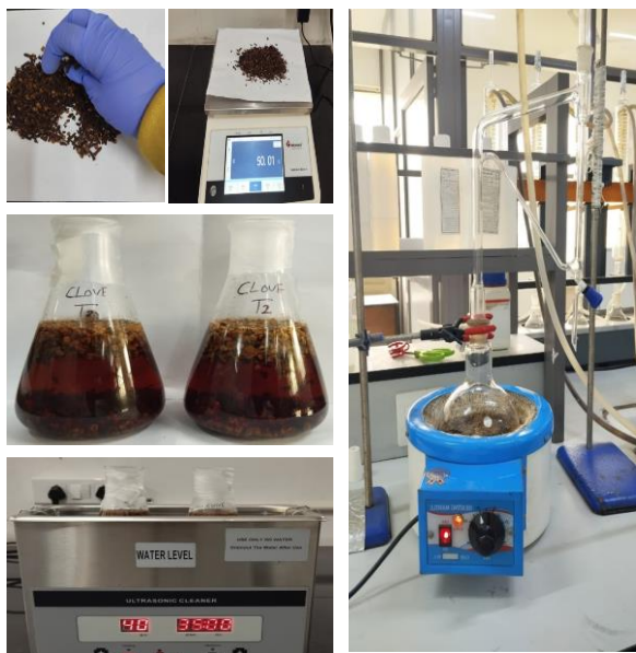
Fig. 1: Process methodology for Ultrasonic Pre-Treated Hydro-distillation system
