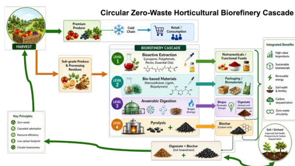
Fig. 2. Circular zero-waste horticultural biorefinery cascade illustrating the four-level valorisation hierarchy from harvest to soil amendment, integrating premium produce cold-chain distribution with cascaded processing of sub-grade produce and residues into bioactive extracts, bio-based materials, bioenergy, and soil amendments, forming a closed-loop circular bioeconomy.
